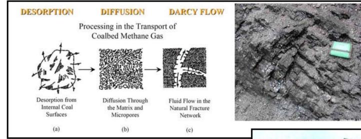
Coal storage (and ECBM) are fundamentally different. Here,  $CO_2$  adsorbs to the organic mineral surface. In doing so, it may liberate  $CH_4$  at ~2:1. The  $CO_2$  is not mobile and does not need to be supercritical.
