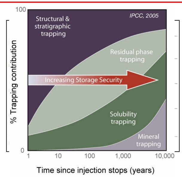
Because of multiple storage mechanisms working at multiple length and time scale, the shallow crust should attenuate mobile free-phase CO<sub>2</sub> plumes, trap them residually, & ultimately dissolve them
