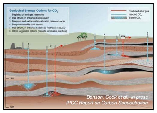
Saline Aquifers Depleted Oil & Gas fields (w/ or w/o EOR and EGR) Unmineable Coal Seams (w/ or w/o ECBM) Other options (e.g., oil shales, basalts)
