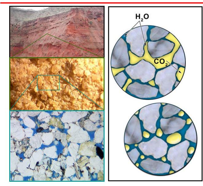
At high pore saturations,  $CO_2$  is mobile and can move as a supercritical phase. At low saturations,  $CO_2$  is trapped by the capillary forces, and will only move by intervention.
