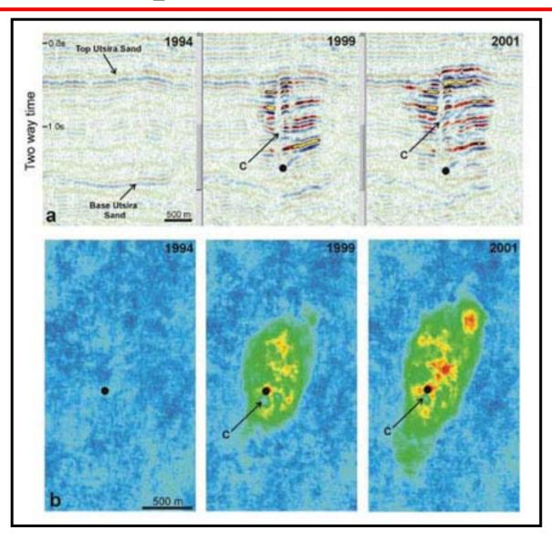
The CO<sub>2</sub> created impedance contrasts that revealed thin shale baffles within the reservoir.
