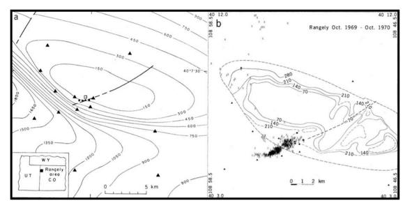
An experiment at Rangely field, CO, attempted to induce earthquakes in 1969-1970. It did so, but only after enormous volumes injected over long times on a weak fault
