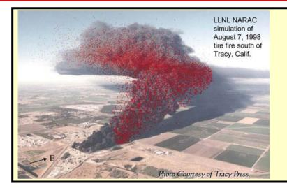
LLNL's NARAC facility is prepared to provide a plume prediction for any location in the US within 15 minutes. It accounts for topography, weather, infrastructure, and calculates risk based on health standards
