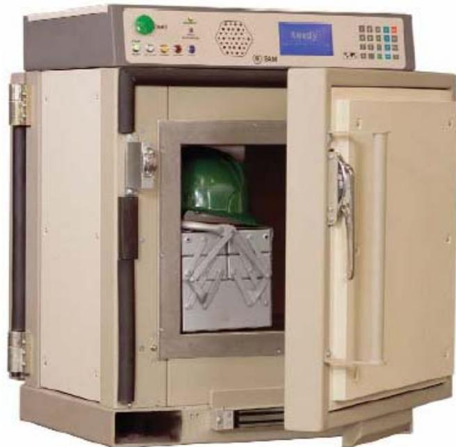
Figure D-1 Example Volumetric Counter (Thermo 2005)
