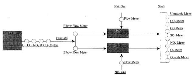
Figure 1. Schematic of Existing and Converted Systems
