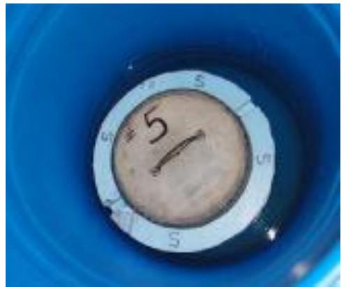
The weight of the Large Area Activated Charcoal Canister (LAACC) unit presses the float into the water creating a seal between the water and the float
