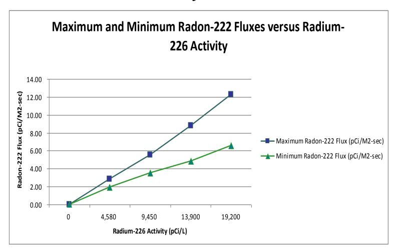
Maximum Slope = 0.00064 Minimum Slope = 0.00034 Average Slope = 0.0004 (previous slide)
