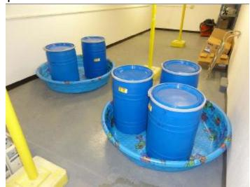
The Radium – 226 in the solutions in the barrels was allowed to attain radiometric equilibrium with the Radon-222 by being allowed to sit covered for forty (40) days (slightly over ten (10) half lives for Radon-222).
