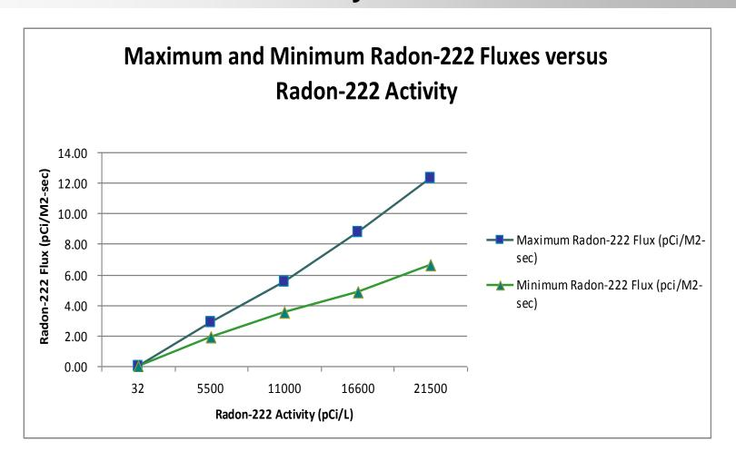
Maximum Slope = 0. 00057 Minimum Slope = 0.00031 Average Slope = 0.0004 (previous slide)
