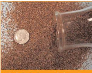
ADA developed and commercialized an arsenic removal POU/POE drinking water system using Amended Silicate<sup>TM</sup> sorbents (pictured above with a dime to indicate scale).
