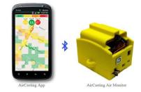
The AirCasting App and Air Monitor enable users to record, map and share health and environmental data using their Smartphone and the portable air monitor. This example and the one below represent types of new technologies available for citizen science activities. EPA encourages new technology development, but does not endorse any products.
