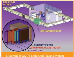
Diagram of AGT's Enhanced Plasma System for Indoor Air Quality, which destroys all types of captured microorganisms while reducing concentrations of airborne VOCs.
