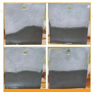
Aluminum 2024-T3 panels prepared with Lynntech conversion coating. No pitting is observed after 336 hours of salt fog spray testing.
