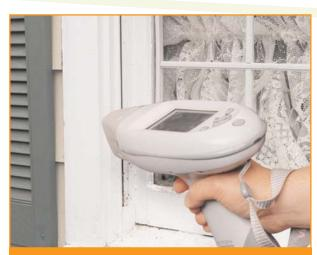
NITON's XLp 300 Series Lead Analyzer, pictured above, can measure the concentration of lead in paint even when covered by 50 or more layers of non-lead paint of unknown thickness and composition.
