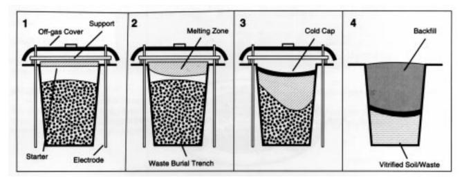
Figure 4. The in situ vitrification operating sequence (USEPA 1990a)
