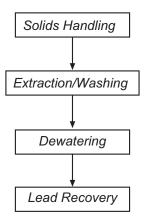
Figure 2. General block diagram of soil washing process
