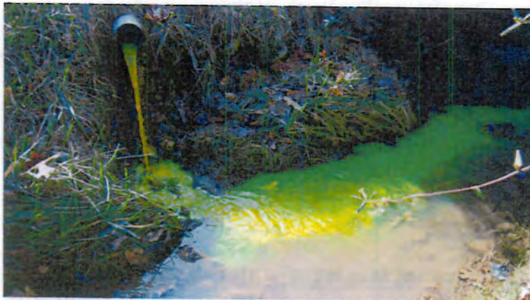
Dye placed in drains, washers, and toilets colors streams and demonstrates that the home's septic system is failing
