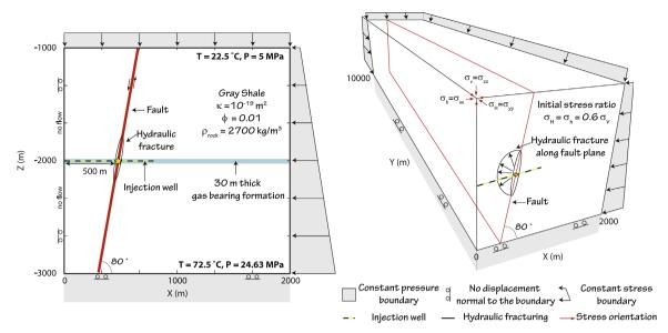
Fig. 1. (Left) 2D-view of the boundary conditions used in the (Right) 3D model geometry for simulating injection and hydraulic fracturing within an 80° dipping fault.
