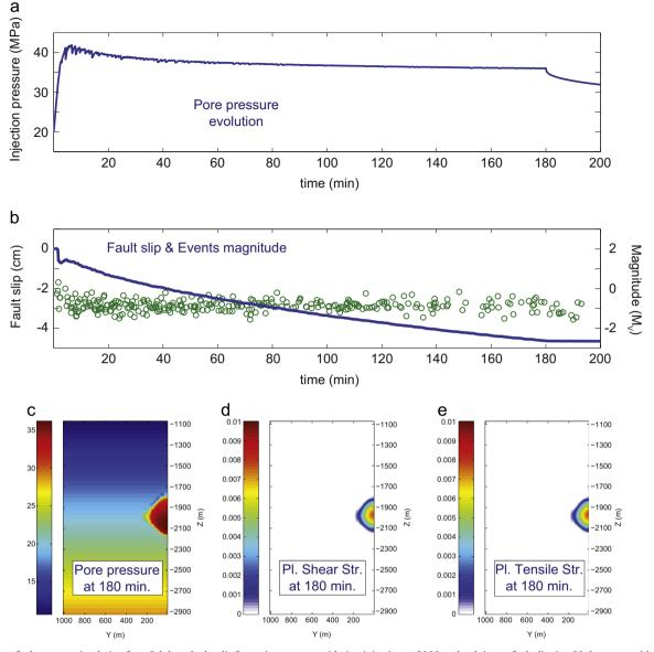
**Fig. 2.** Results of a base-case simulation for a 3-h long hydraulic fracturing stage considering injection at 2000 m depth into a fault dipping 80 degrees, and having a peak coefficient of friction of 0.6 and a residual friction of 0.4: (a) Downhole well pressure and (b) fault slip and events moment magnitude as function of time, and (c to e) pore pressure, plastic shear strain (signifying shear slip), and plastic tensile strength (signifying tensile failure) at the end of the 3-h injection.
