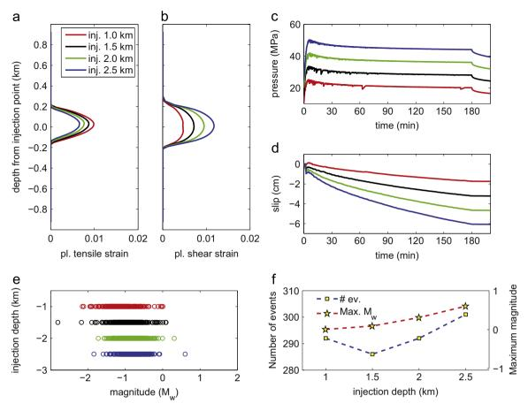
**Fig. 3.** Sensitivity of simulation results to changes in injection depth: Vertical extent of (a) plastic tensile strain (signifying tensile failure) and (b) plastic shear strain (signifying shear slip), and time evolution of (c) well pressure and (d) slip magnitude, and (e) magnitude distribution for each value of injection depth and (f) number of events and maximum magnitude as a function of the injection depth.
