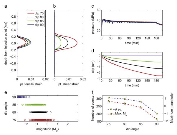
**Fig. 4.** Sensitivity of simulation results to changes in fault dip: Vertical extent of (a) plastic tensile strain (signifying tensile failure) and (b) plastic shear strain (signifying shear slip), and time evolution of (c) well pressure and (d) slip magnitude, and (e) magnitude distribution for each dip angle and (f) number of events and maximum magnitude as a function of fault dip angle.
