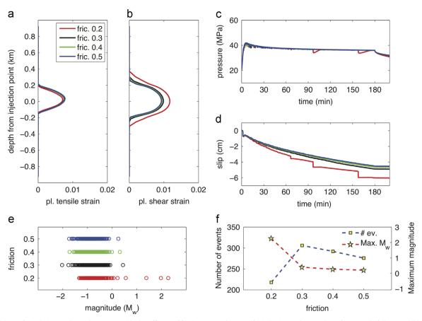
**Fig. 6.** Sensitivity of simulation results to changes in residual coefficient of friction: Vertical extent of (a) plastic tensile strain (signifying tensile failure) and (b) plastic shear strain (signifying shear slip), and time evolution of (c) well pressure and (d) slip magnitude, and (e) magnitude distribution for each value of the residual friction and (f) number of events and maximum magnitude as a function of residual coefficient of friction.
