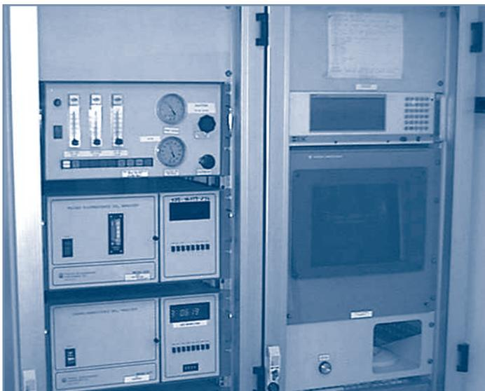
CEM monitor for SO<sub>2</sub>, NO<sub>x</sub> and CO<sub>2</sub>
