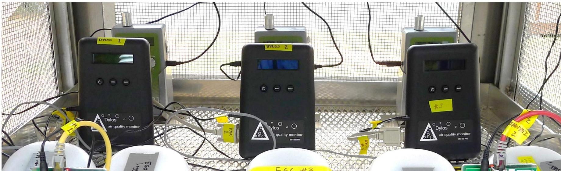
Figure A-3. Dylos units inside the chamber (Figure A-1) during field deployment.
