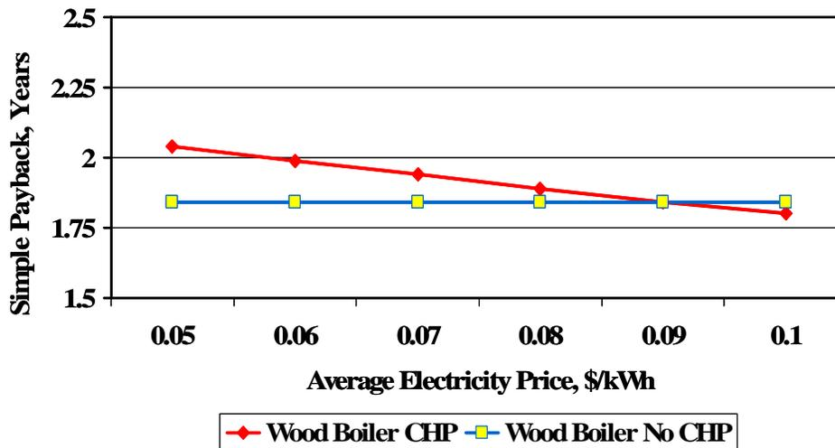
Figure 4 shows the sensitivity of the annual operating cost savings to the average price of displaced electricity for the wood boiler/steam turbine CHP system 1 and for the wood boiler/no CHP system (both based on \$15.00/ton purchased wood costs). Annual cost savings increase significantly for the CHP system with rising electricity prices. Annual operating cost savings at \$0.09/kWh are \$10,400,000 for the CHP case compared to \$8,500,000 for the wood boiler/no CHP option.
