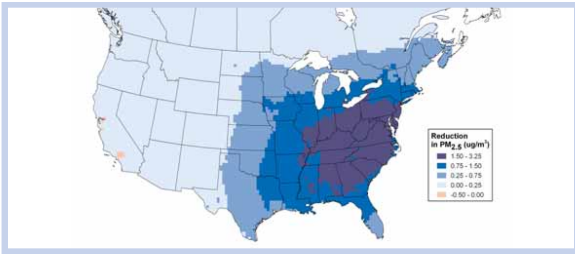
Figure H-17 Absolute Change in Annual Fine Particles ( \mu\text{g}/\text{m}^3 ) with Emission Reductions under Illustrative Trading Scenario Compared to the Base Case in 2020 (CMAQ)
