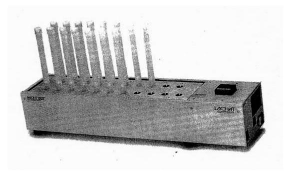
Figure 4 MICRODIST DISTILLATION TUBE
