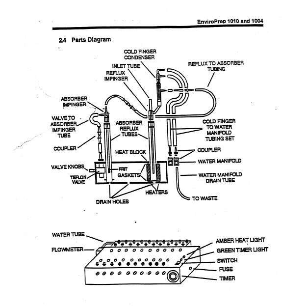
Figure 3 MICRODIST DISTILLATION DEVICE
