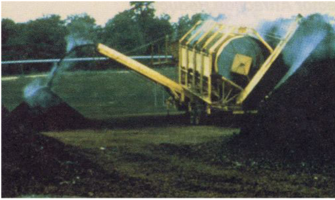
Composted sludge is screened to remove the bulking agent prior to land application
