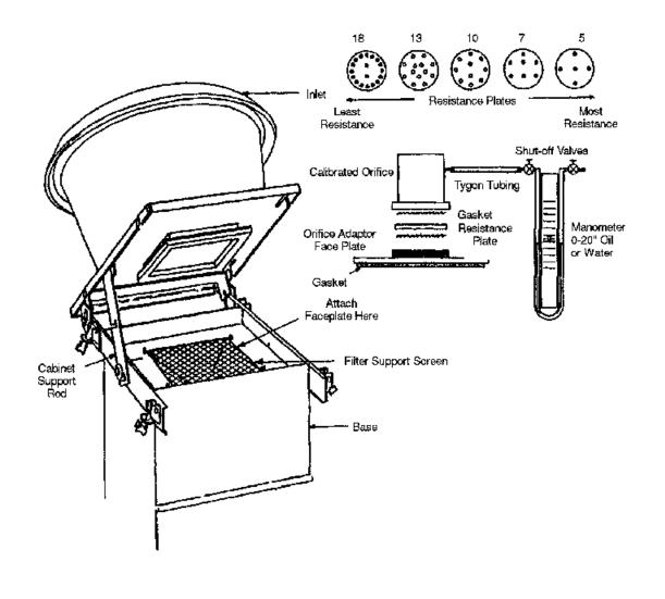
Figure 10. Typical calibration set-up for a mass flow controller (MFC).
