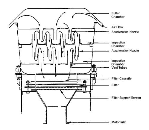
Figure 4. Schematic diagram of an impaction inlet for size select sampling for particulate matter.
