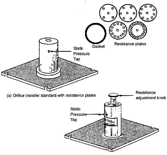
(b) Variable resistance orifice transfer standard
