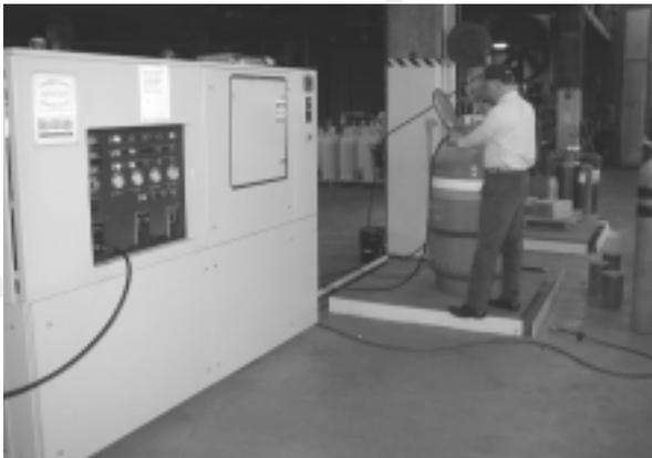
Technician connecting hose to a halon storage cylinder from a halon recycling unit operated in accordance with NFPA standards. EPA regulations prohibit disposal of halon except by sending it for recycling to a recycler operating in accordance with NFPA standards – or by arranging for its destruction via approved processes. Photo courtesy of U.S. DOD/DLA ODS Reserve.
