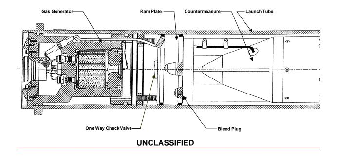
Figure 2. Location of Countermeasures Launcher Components Within a Launch Tube
