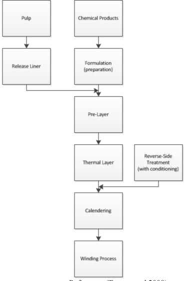
Figure 5-3: The Production Process for Thermal Paper
