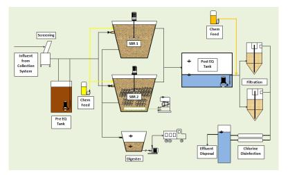
control the batch time, which had been targeted to be 4 hours, but could be longer if flows were insufficient or shorter if there was a hydraulic surge (e.g., from a storm event). Each batch includes a fill cycle, react cycle, settle cycle, decant/waste activated sludge (WAS) cycle, and idle cycle.
