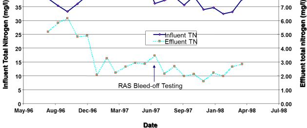
The figure below shows how the RAS bleed-off and associated increase in mixed liquor suspended solids (MLSS improved denitrification within the secondary anoxic zones. In the Blue Heron WRF, the MLSS concentration of the secondary anoxic zone was increased by about 20 percent, while the average effluent TN was reduced by nearly one-half during the test period profiled.
