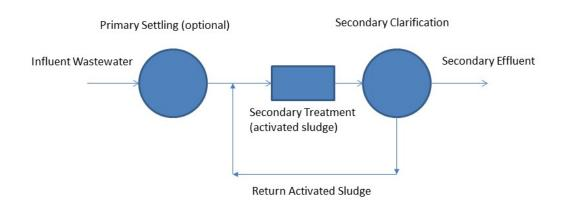
Figure 2-6. Basic (non-advanced) Activated Sludge WWTP process schematic
