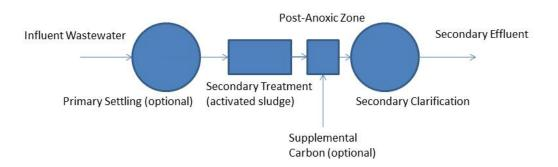
Figure 2-3. Generalized post-anoxic zone nitrification/denitrification liquid-phase treatment schematic
