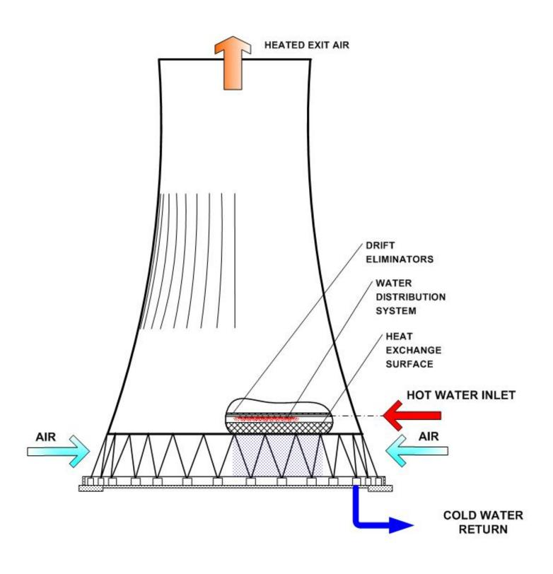
Figure 2-2: Typical Natural Draft Cooling Tower Schematic
