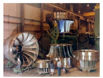
Figure 5–14. New Replacement Runners from 1 to 194 MW. (Source: American Hydro).
