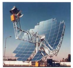
Figure C-4. Parabolic Dish Receiver (Source: Stirling Energy Systems).
