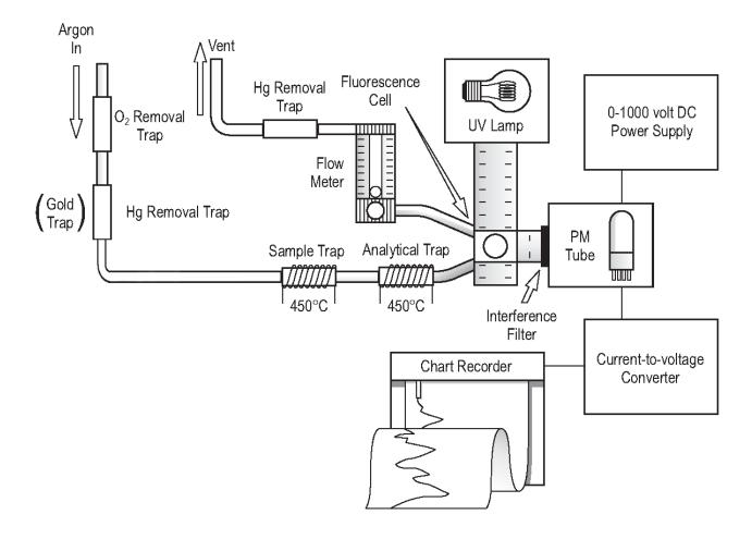
Figure 2. Schematic Diagram of the Bubbler, Purge and Trap, Cold Vapor Atomic Fluorescence Spectrometer (CVAFS) System
