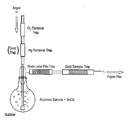
Figure 1. Schematic Diagram of Bubbler Setup
