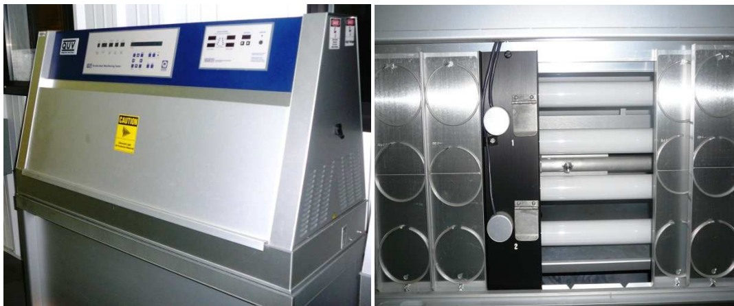
Figure 2.10. QUV Accelerated Weathering Tester: exterior (left); UV lamps (right)
