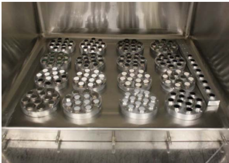
Figure 2.5. Sample stages in the test chamber
