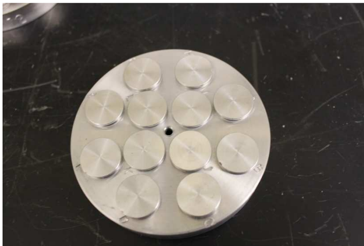
Figure 2.4. Sample stage with aluminum pin mounts
