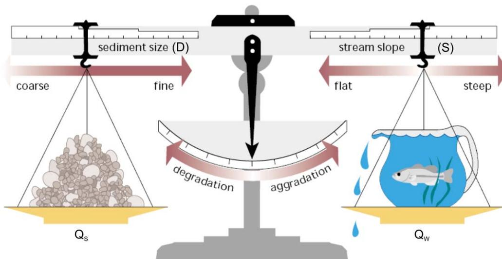
Figure 2.2 Factors Affecting Channel Degradation and Aggradation (FISRWG, 1998)
