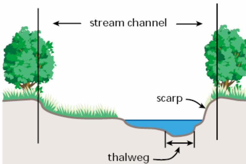
Figure 2.1 Cross-section of a Stream Channel (FISRWG, 1998)
