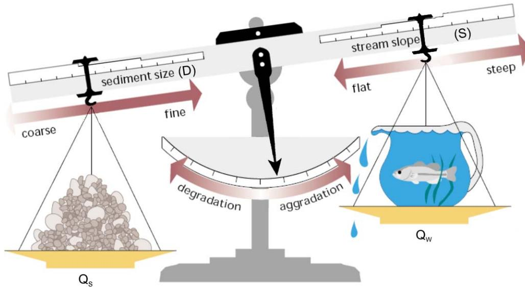
Figure 2.3 Example of Aggradation (Adapted from FISRWG, 1998)
