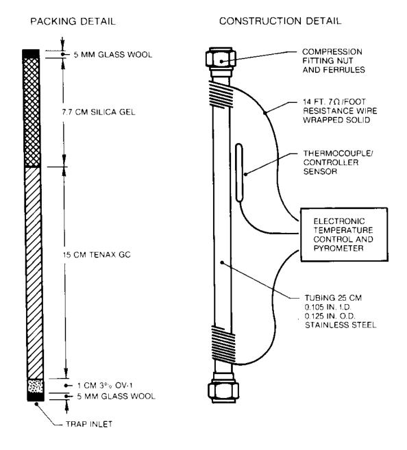
FIGURE 3 Trap Construction and Packings
