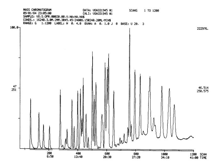
FIGURE 9 Chromatogram of Aqueous Performance Standard
