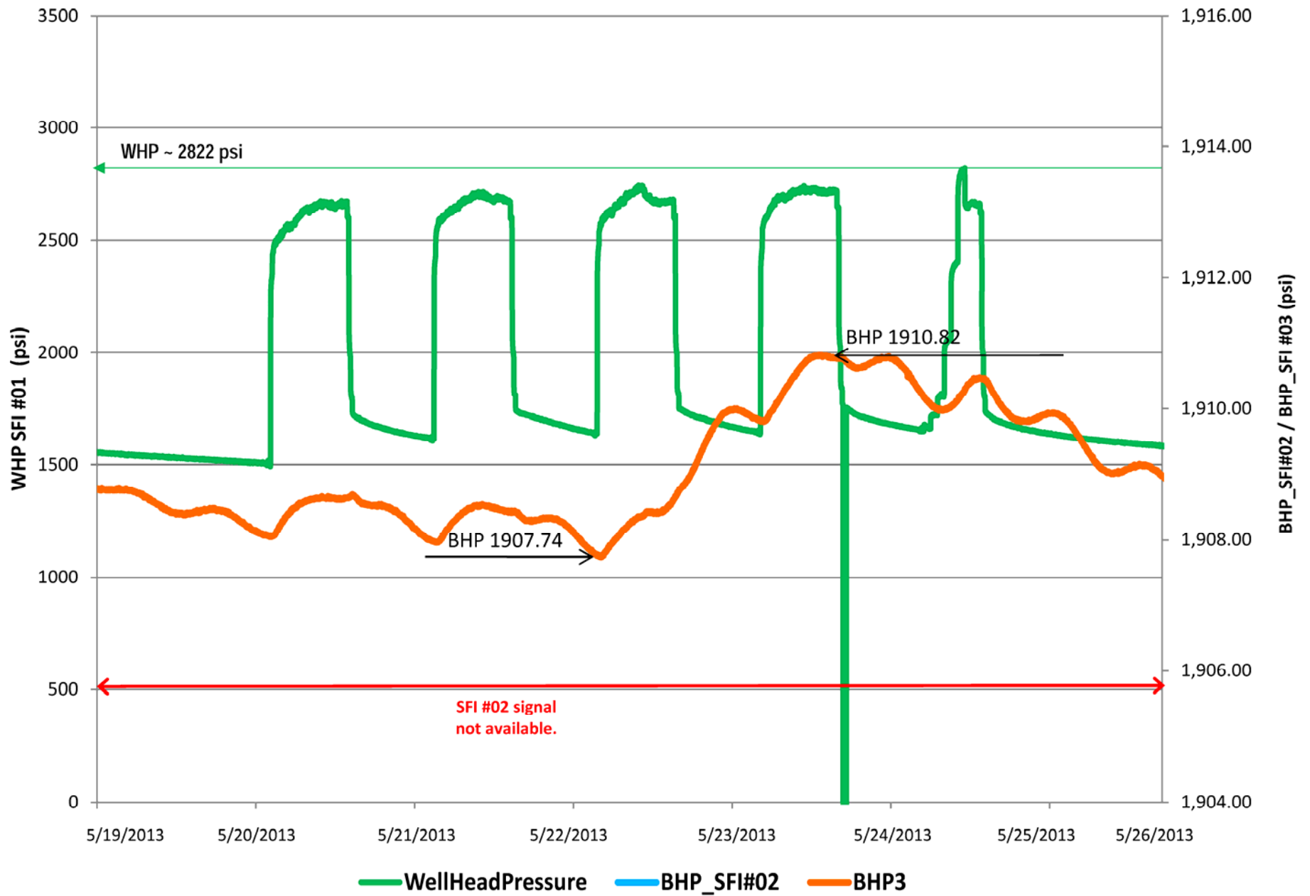
Figure 2 – SFI#2 and SFI#3 Bottom-Hole Pressure Data for Week of May 19 thru May 26, 2013
