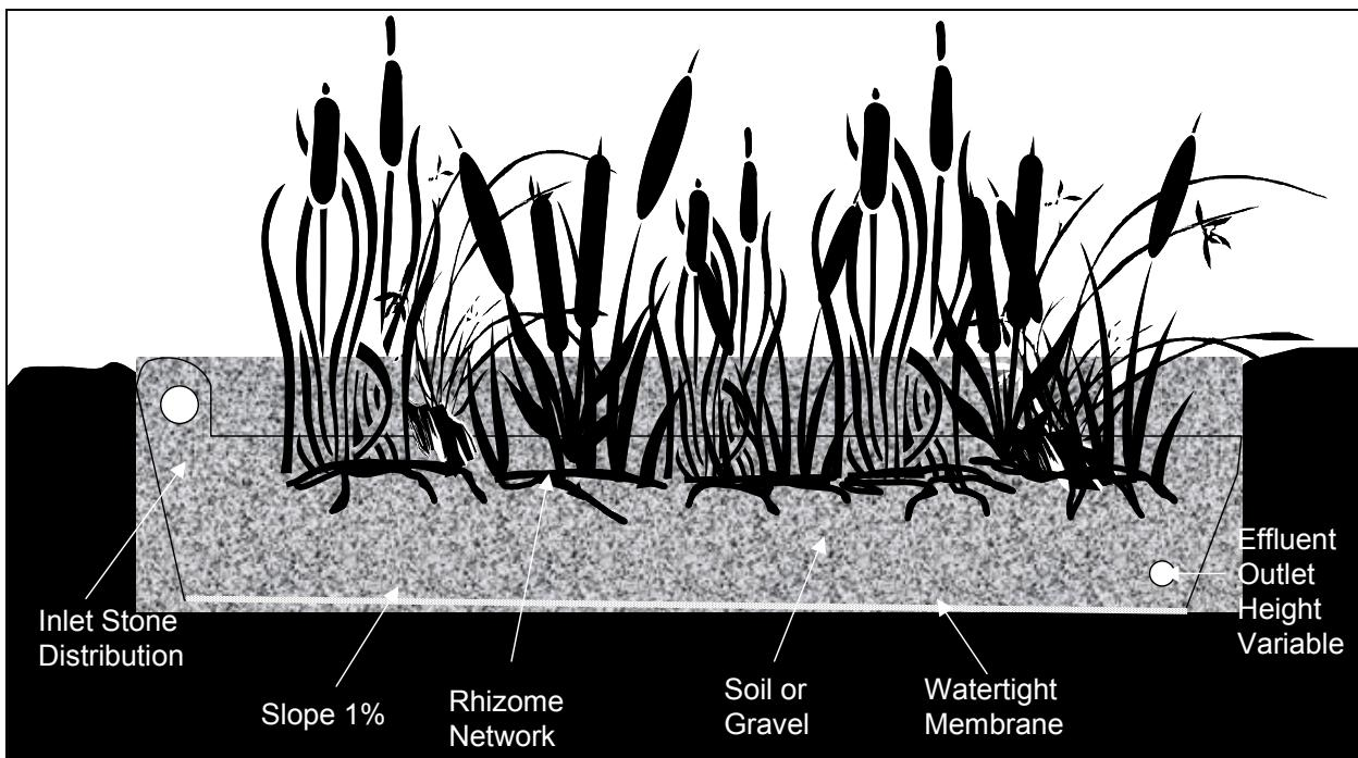
**Figure 6.5: Components of a vegetated submerged bed.**
