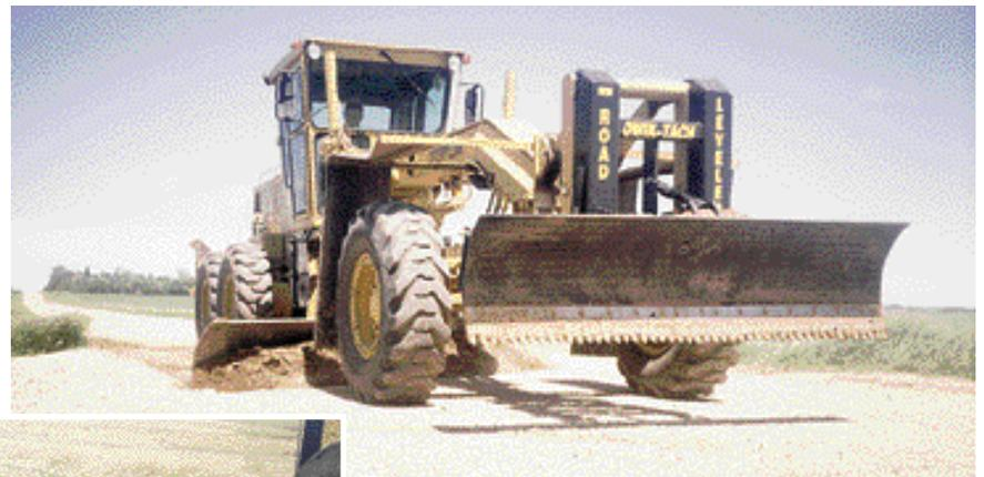
This dozer blade is also equipped with carbide bits which allows the operator to use it for particularly hard cutting such as taking out washboard areas on the road. The operator then uses the grader's moldboard with a conventional cutting edge to shape the area.
