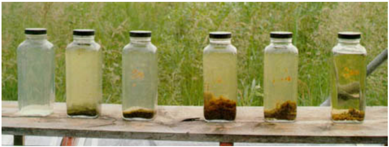
Bottles with representative samples (taken from the influent [on left] to final [on right] sample stations) from the Houghton Lake, MI, wetland treatment system which has been in operation since 1978.
