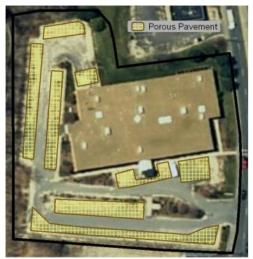
Figure 3A3-8. Actual site and on-site control measures (Boston, MA).
