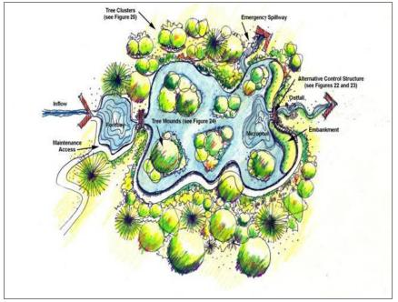
Source: VA DCR 2009 Figure 3A1-23. Plan view constructed wetland basin.
