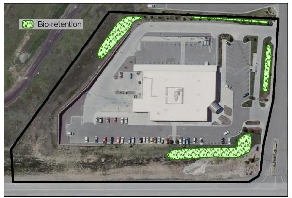
Figure 3A3-4. Actual site and on-site control measures (Denver, CO).
