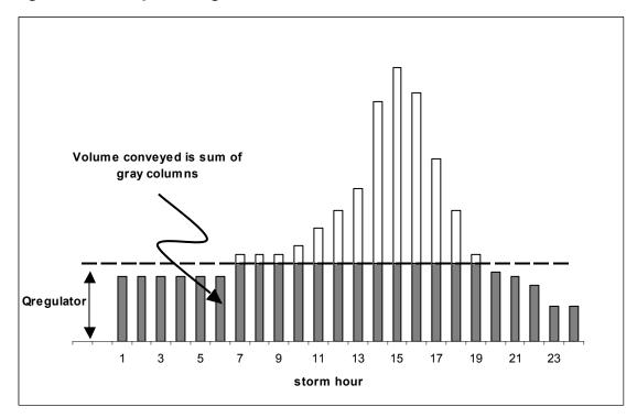
Figure 3. Conceptual Diagram of Calculation of Fraction Diverted
