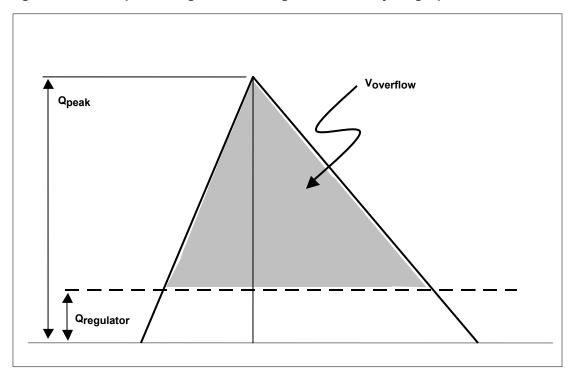
Figure 1. Conceptual Diagram of Triangular Runoff Hydrograph
