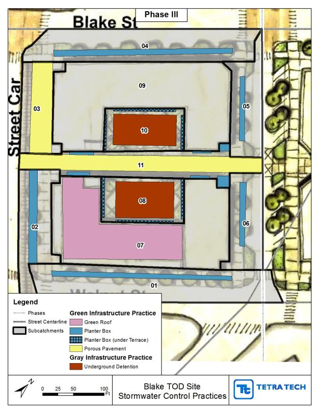
Figure 20. Phase III Stormwater Control Measure Layout.
