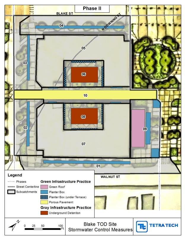
Figure 19. Phase II Stormwater Control Measure Layout.
