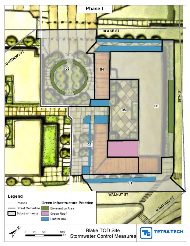
Figure 18. Phase I Stormwater Control Measure Layout.
