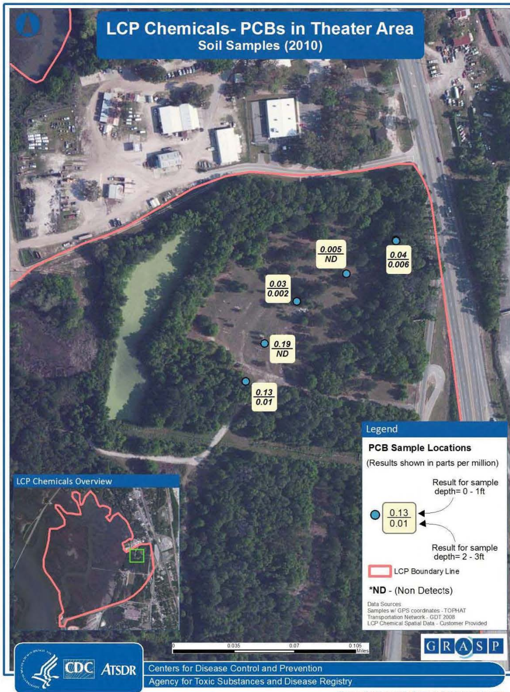
Figure 14. Sampling Locations Showing Concentration of PCBs in Soil In Theater Area, 2010
