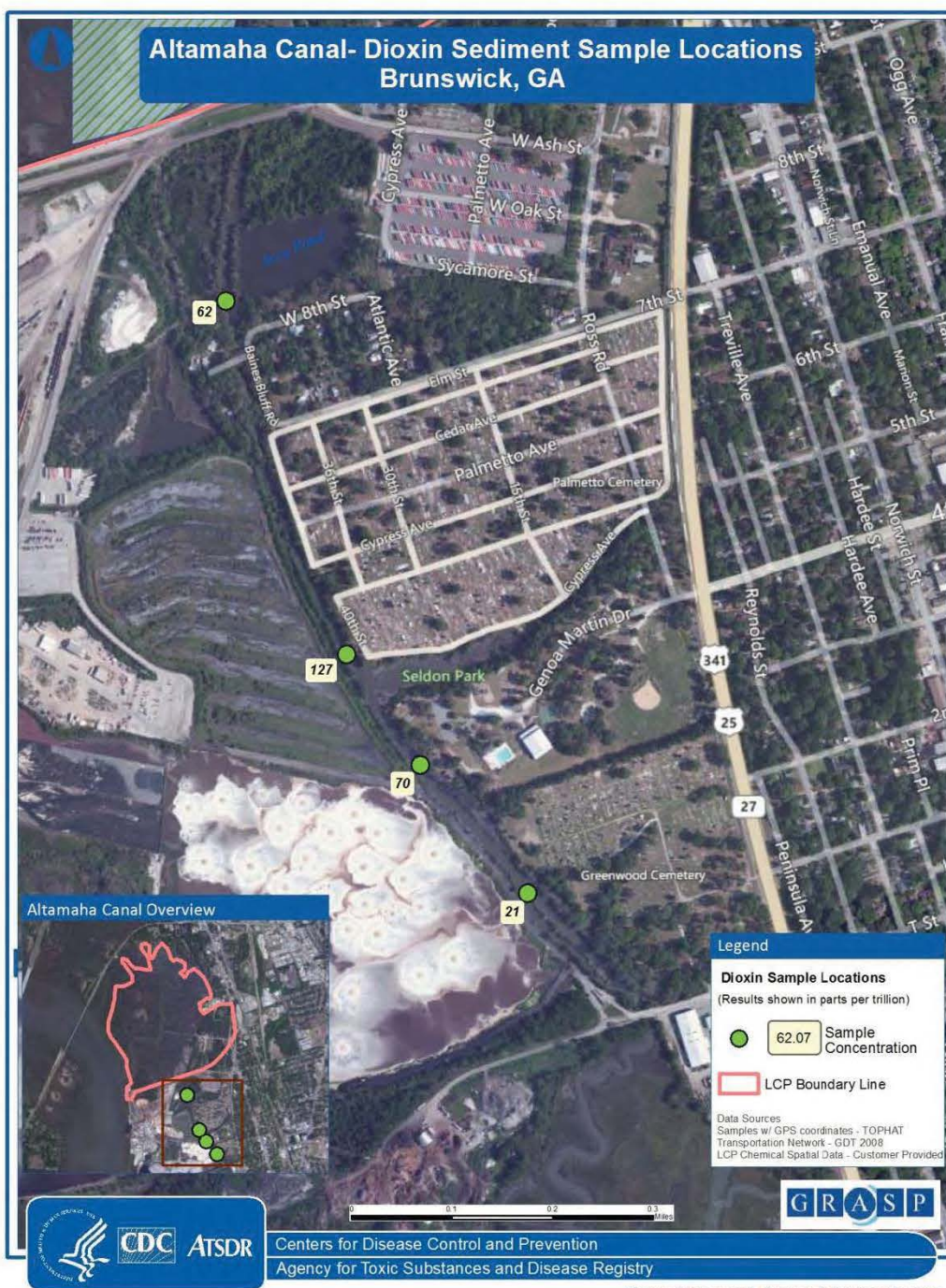
Figure 30. Sampling Locations Showing Concentration of Dioxins in Sediment in Altamaha Canal, 2011 Just South of the LCP Chemicals Site.
