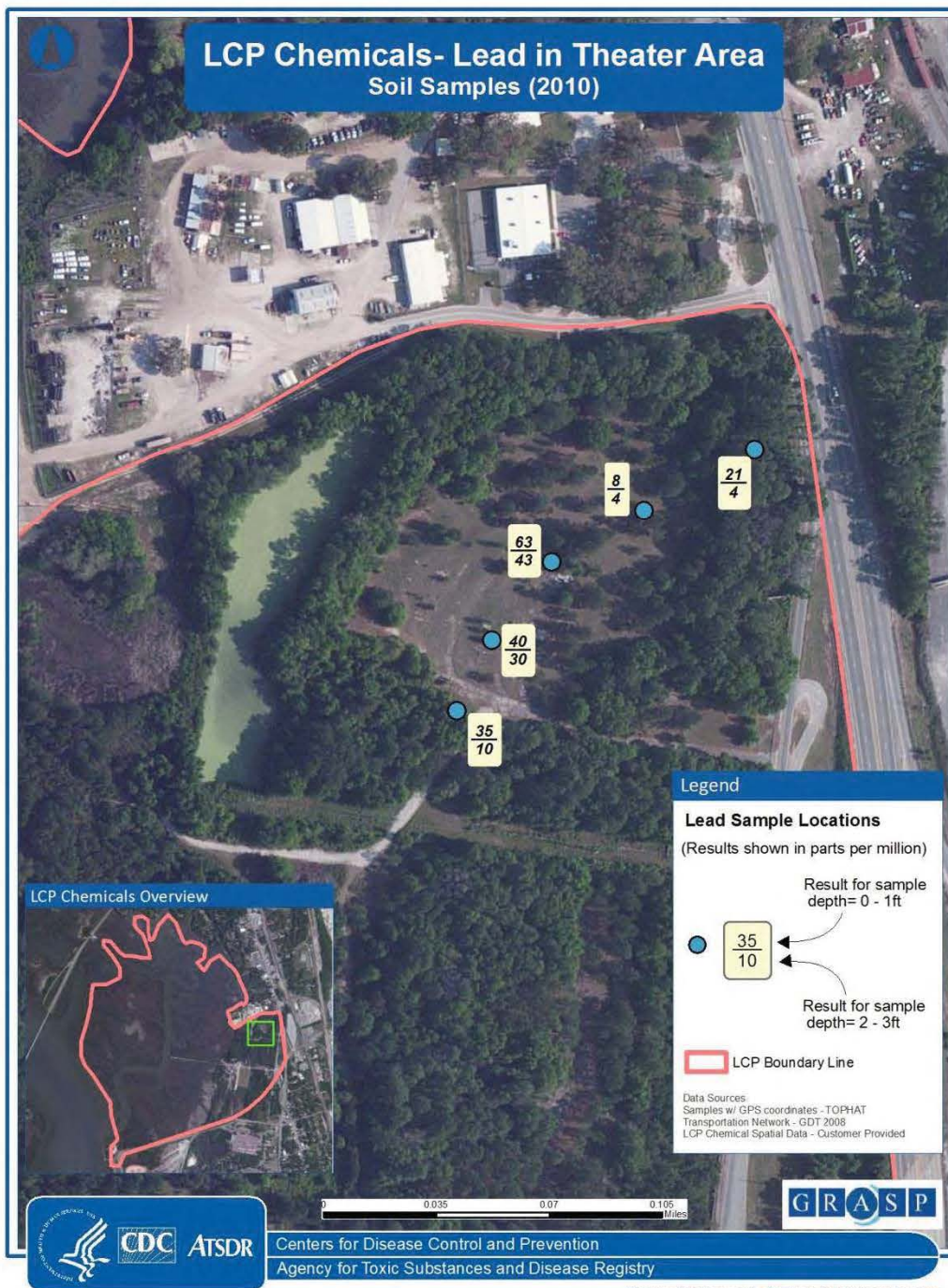
Figure 17. Sampling Locations Showing Concentration of Lead in Soil In Theater Area, 2010
