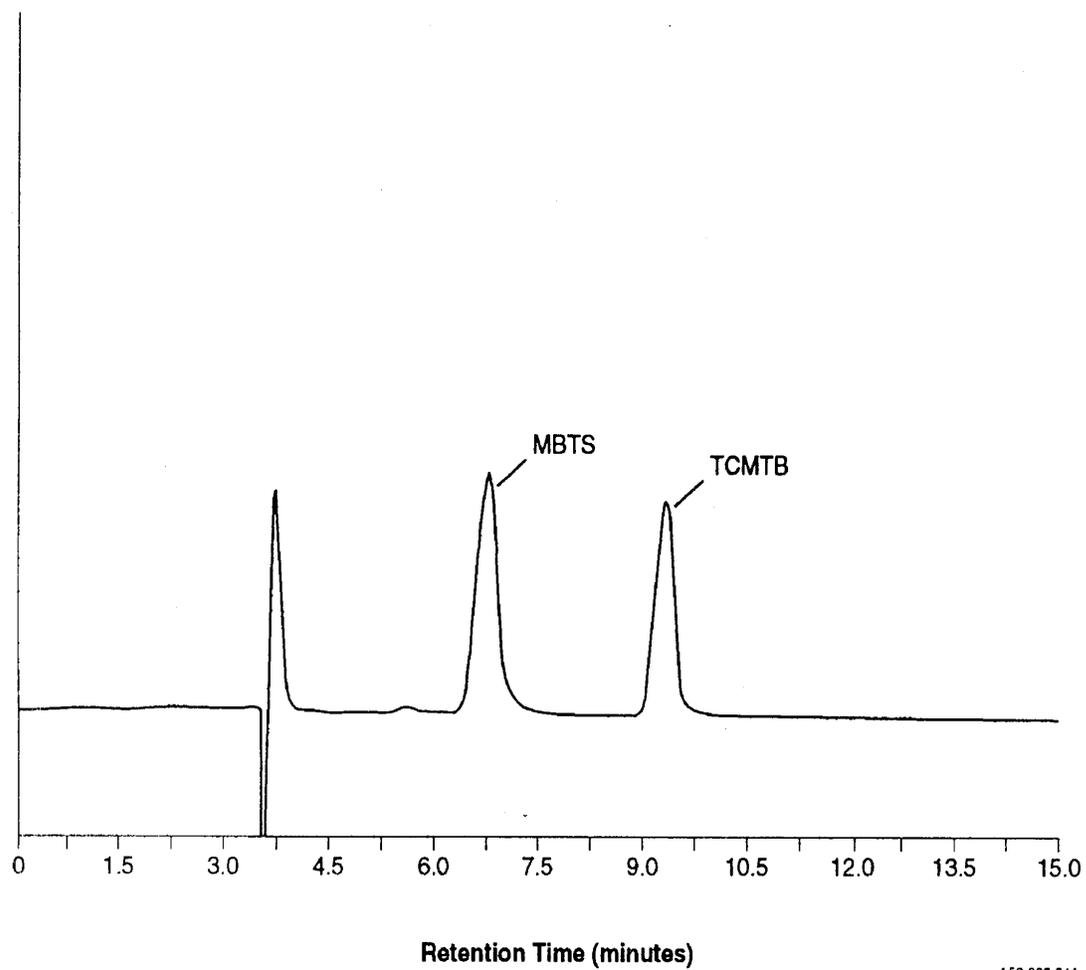
Figure 1. HPLC-UV Chromatogram of 10 ng Each of MBTS and TCMTB (Column 1)
