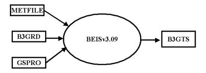
Figure 2. The program beis3 input data flows
