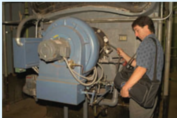
Jamie Harvey uses a Lumex unit to test for mercury at an industrial site.
