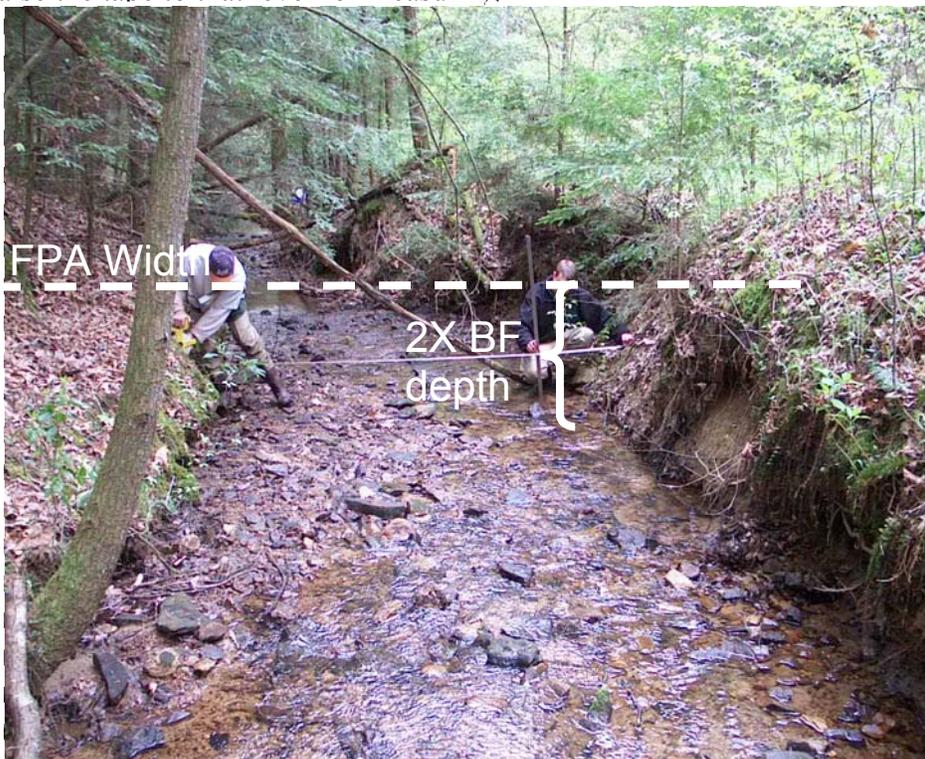
**Figure 3-39** Photograph illustrating flood-prone area (FPA) width.
