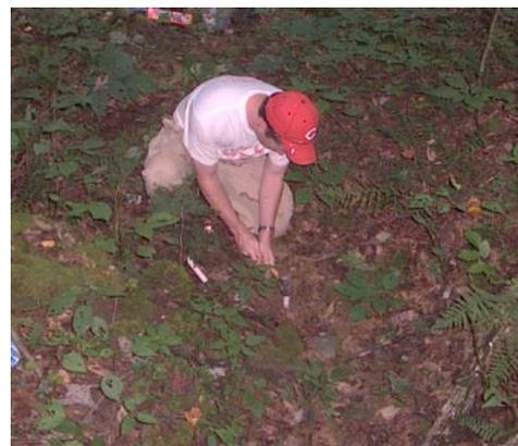
**Figure 3-55 Tapping core vertically into streambed.**
