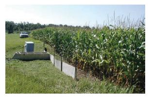
Edge-of-field runoff monitoring equipment
