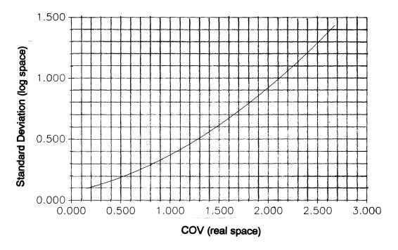
Figure 5. Relationship between standard deviations (log<sub>10</sub> space) and coefficient of variation (real space).
