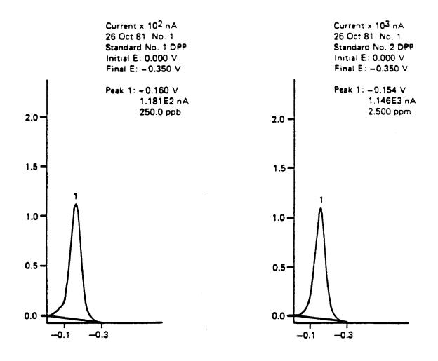
Figure 2. Typical differential pulse polarogram at 0.25 ppm and 2.5 ppm Cr in 0.1 N buffer.
