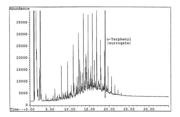
FIGURE 3  ${\rm EXAMPLE~CHROMATOGRAM~OF~A~30~PPM~DIESEL~STANDARD~WITH~THE~} \\ {\rm BASELINE~PROJECTED~BETWEEN~C_{10}~AND~C_{28} }$
