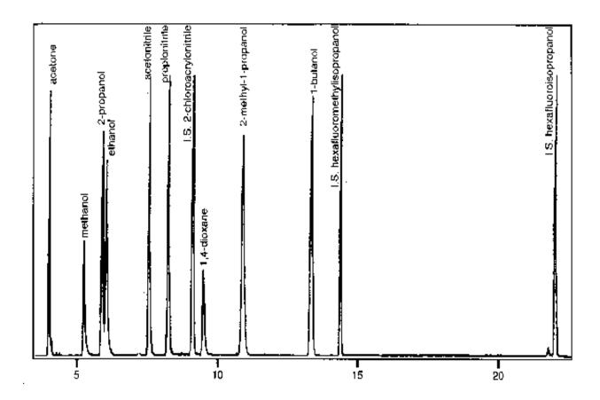
Mix 1: Analytes distilled at 0.25 mg/L, internal standards at 2.5 mg/L
