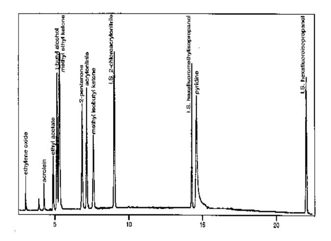
Mix 2: Analytes distilled at 0.25 mg/L, internal standards at 2.5 mg/L
