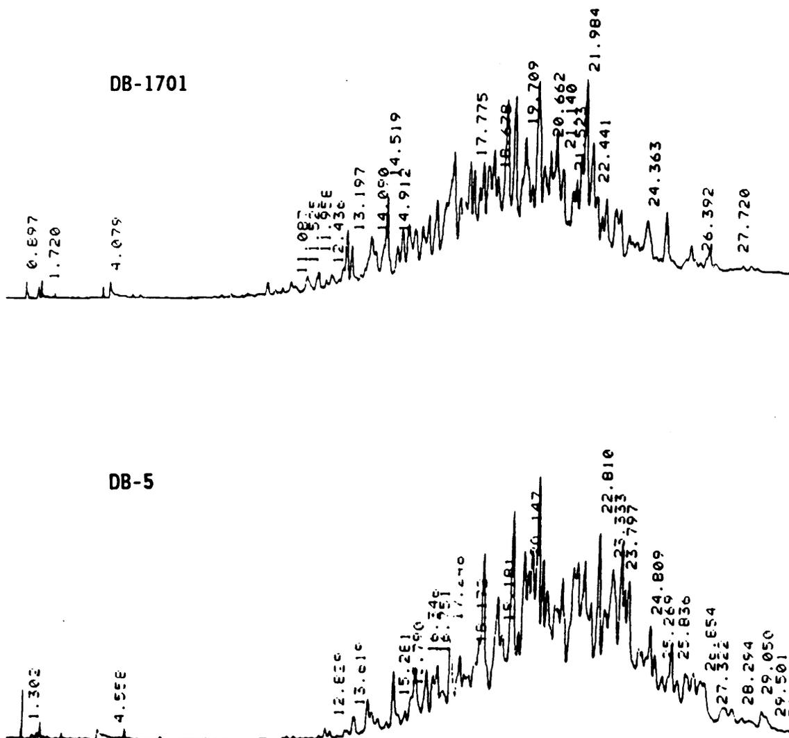
Strobane analyzed on a DB-5/DB-1701 fused-silica open-tubular column pair. The GC operating conditions were as follows: 30-m x 0.53-mm ID DB-5 (1.5- $\mu$ m film thickness) and 30-m x 0.53-mm ID DB-1701 (1.0- $\mu$ m film thickness) connected to a J&W Scientific press-fit Y-shaped inlet splitter. Temperature program: 150 °C (0.5 min hold) to 190 °C (2 min hold) at 12 °C/min then to 275 °C (10 min hold) at 4 °C/min.
