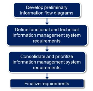
Figure 4-4. Process for Developing Information Management System Requirements
