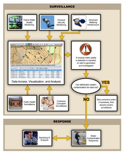
Figure 1-1. Surveillance and Response System Components
