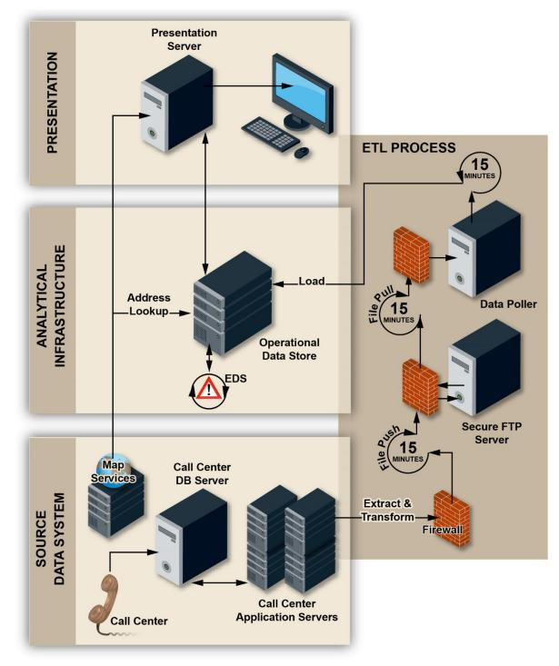
Figure 4-9. Example of a CCS Physical Architecture Diagram
