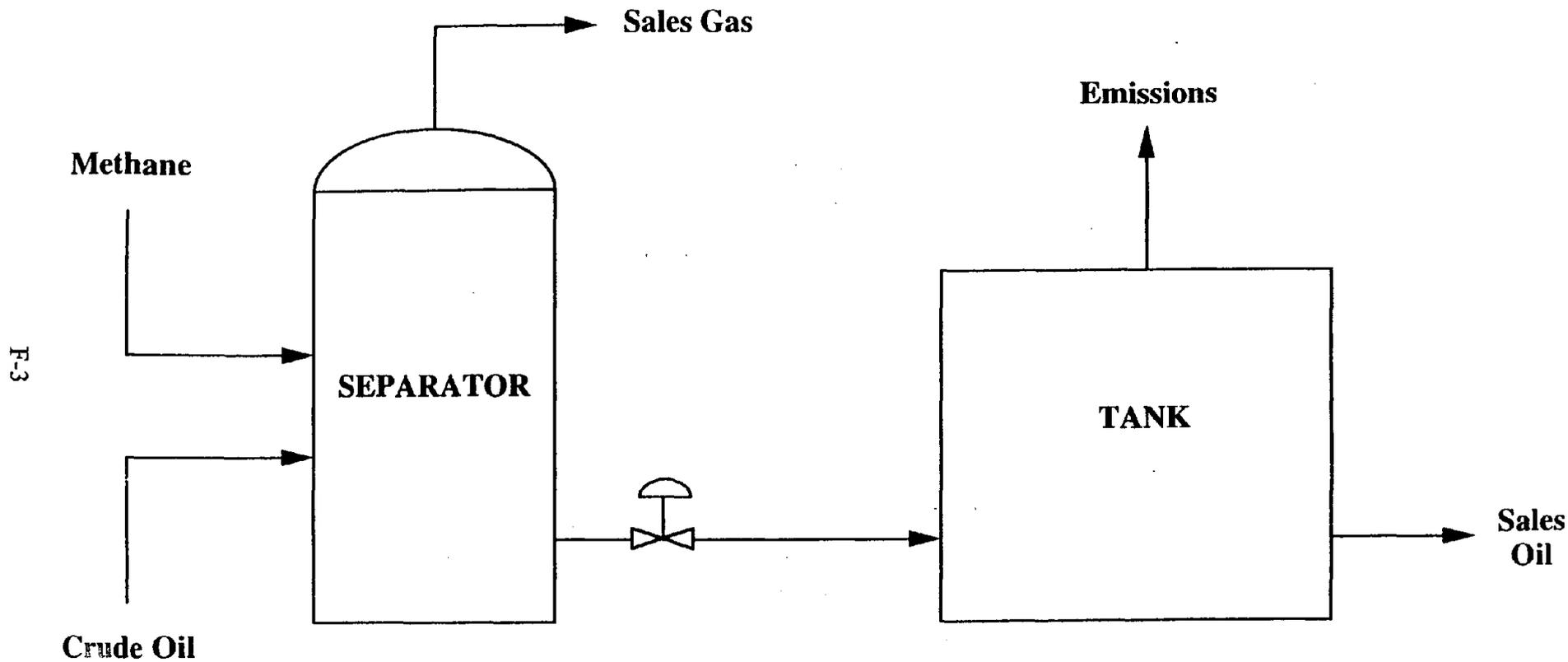
**Figure F-1. Process Flow Diagram for Simulations to Determine Methane Emissions from Oil/Condensate Production Tanks**
