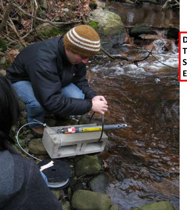
DATASONDES MEASURE TEMPERATURE AND SPECIFIC CONDUCTIVITY EVERY 15 MINUTES
