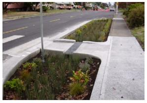
Figure 6. This landscaped curb extension demonstration project, located on at the intersection of 131st and Freemont Streets, shows how these features can be easily adapted to allow for pedestrian traffic.
